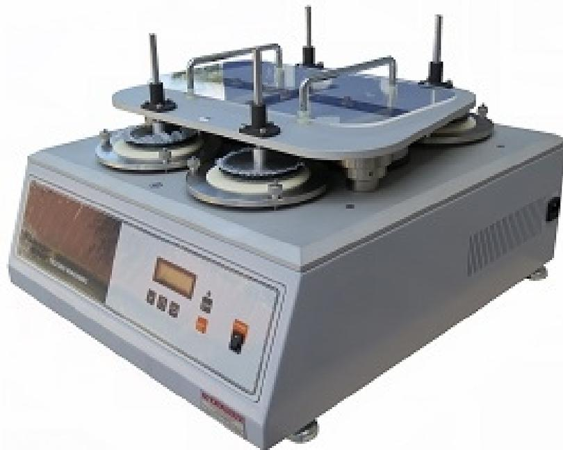
PERMET DE DETERMINER LE NIVEAU D'ABRASION
